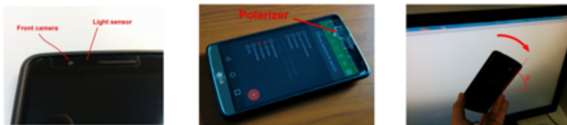
Figure 4: Example of mounting of the polarizing lens on the light sensor and performing the experiment.
