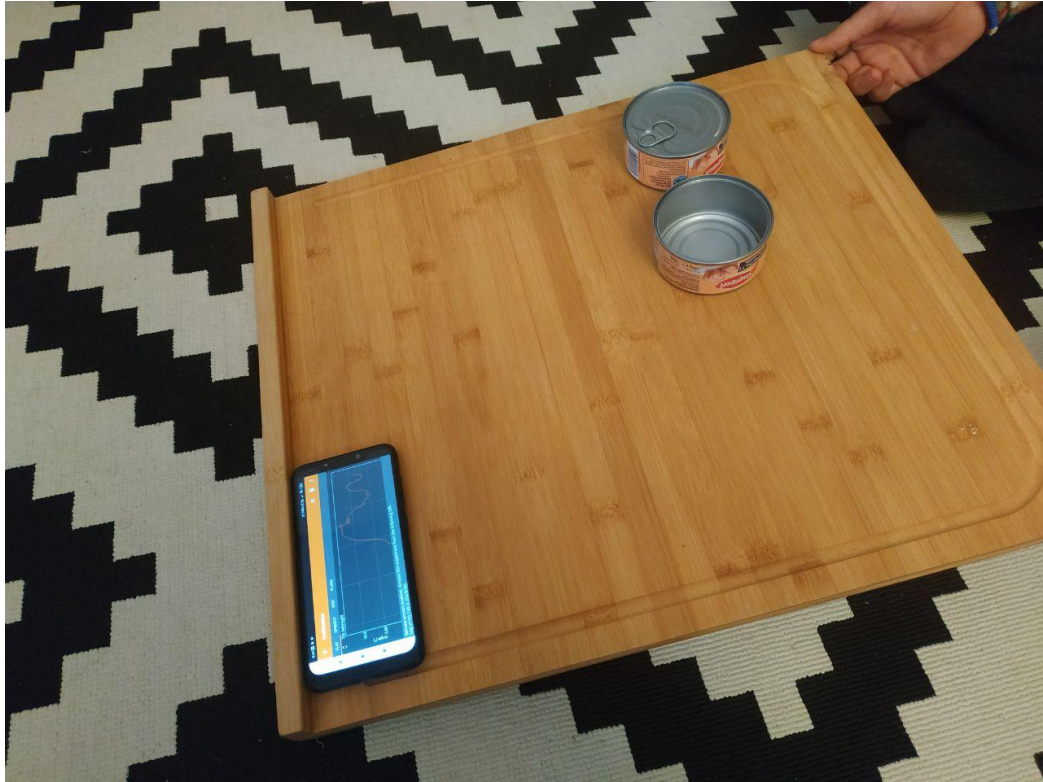
Figure 2: Setup to measure the friction coefficient
