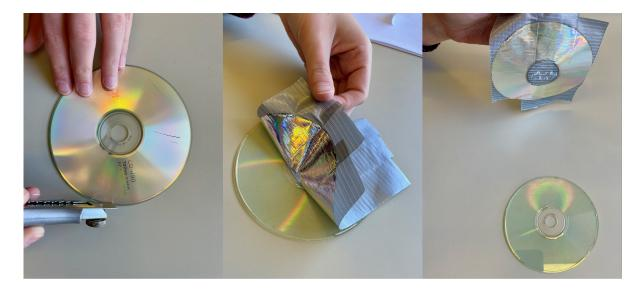
The goal is to remove the silver foil from the CD and reveal the transparent part with the tiny grooves that will act as a diffraction grating. In order to do that:
