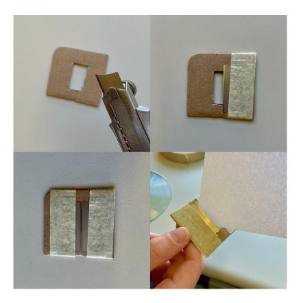
This is the step that requires the most precision, as we need to create a slit with smooth edges which are parallel to each other, and which are separated by about 0.1 mm. Perform the following steps:
