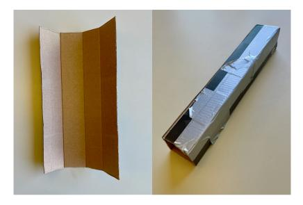
The dimensions of the tube (box) do not affect the results significantly. You can pick any reasonable shape and size. However, the material used is of importance, especially the inner surface - ideally it should not reflect light and should be rather dark.
